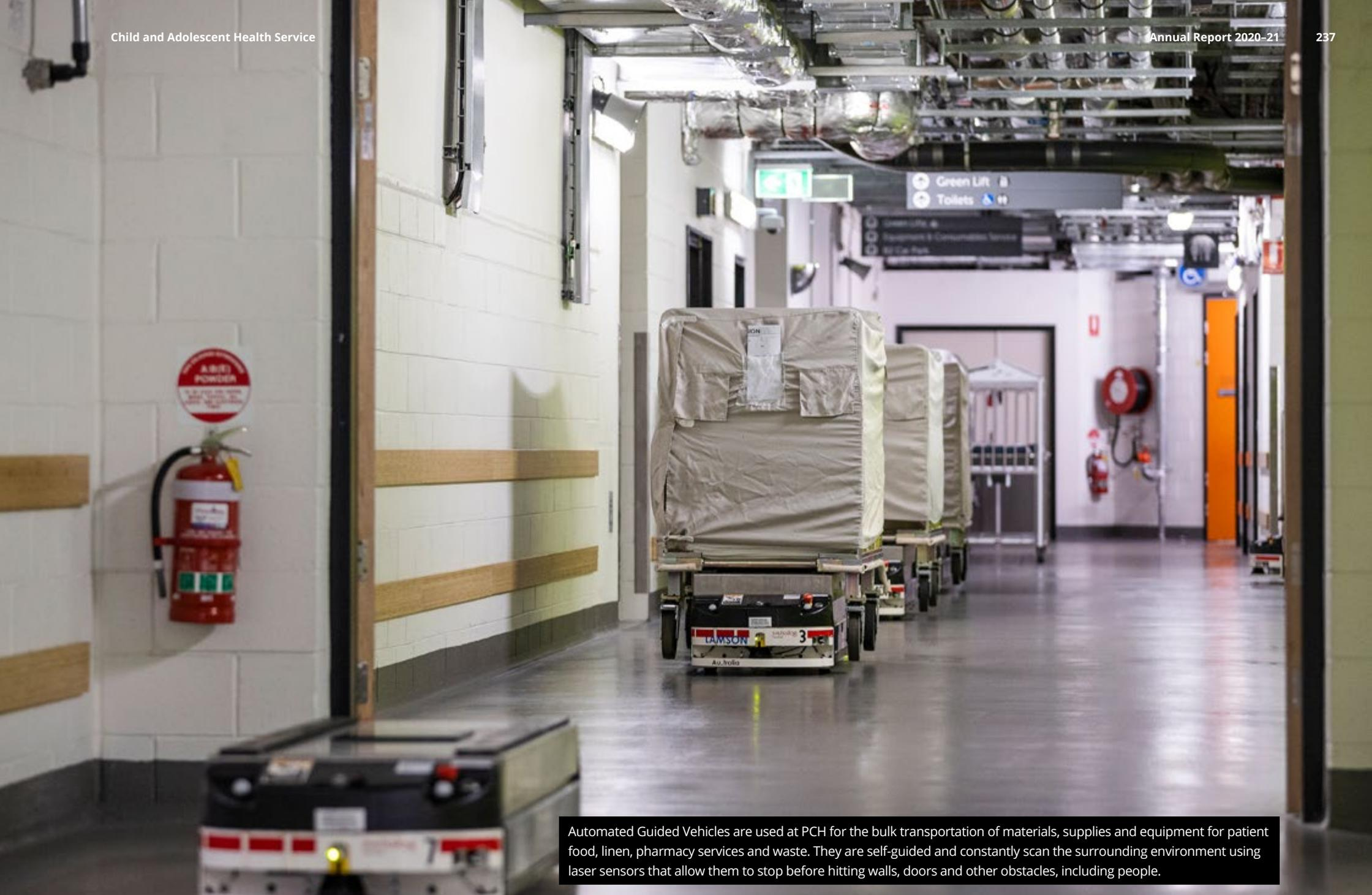
Automated Guided Vehicles are used at PCH for the bulk transportation of materials, supplies and equipment for patient food, linen, pharmacy services and waste. They are self-guided and constantly scan the surrounding environment using laser sensors that allow them to stop before hitting walls, doors and other obstacles, including people.
